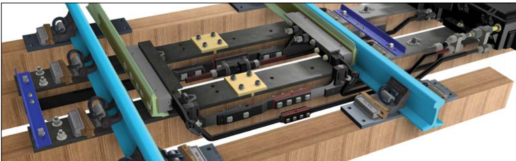
Typical Dual Point Detection Layout
