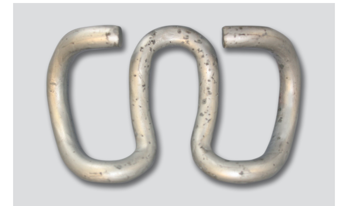
After 1440 h in the salt spray test according to ISO 9227 NSS with intentional layer damage to demonstrate the cathodic corrosion protection.
