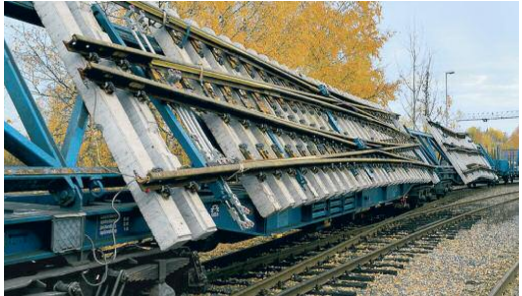
With a new Vossloh concept, switches in Sweden can now be changed much more quickly—within eight hours.
