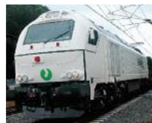
EURODual—also runs on trackage with overhead wires
