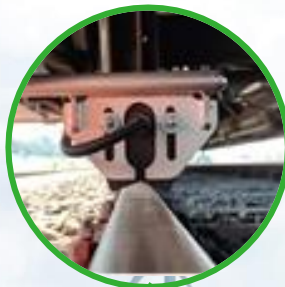
Longitudinal profile measurement using laser sensors
