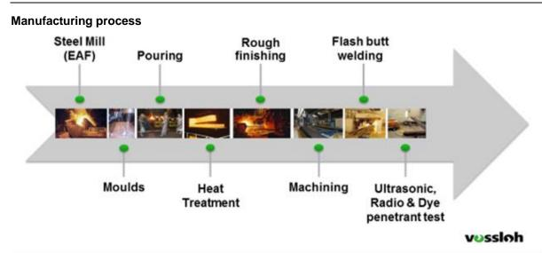
All cast manganese products have the same grade that could answer to many technical specifications. Manganese steel is 100% recyclable after use in service even after many years. It means that we can always melt "recycling" crossings in our furnace and manufacture new crossings.
