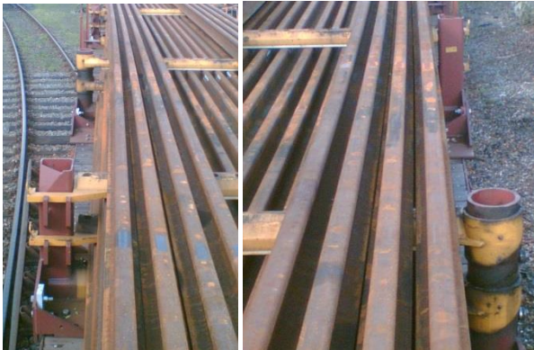
Without locking pins: rails free to slide
