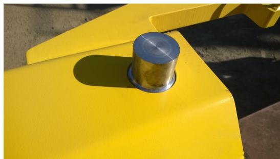
Locking pin in a rail support arm
