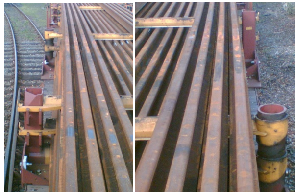
Without locking pins: rails slide freely
