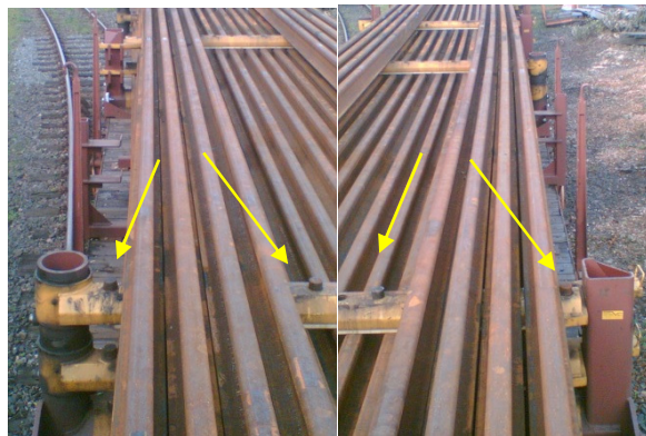
Locking pins above bogie: rails laterally restrained
