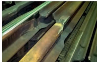
Transition between grooved rail and flange rails
