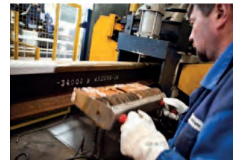
Numerical identification for tracking each weld joint
