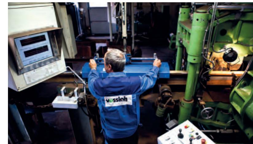
After welding comes straightening and refining
