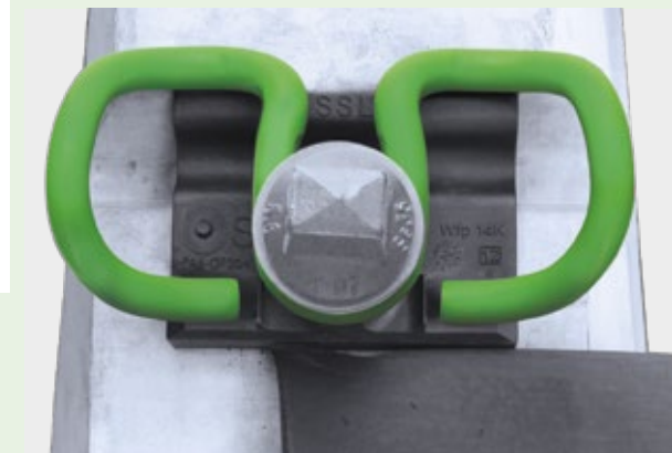
Rail pad after strong longitudinal movement of rail
